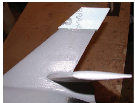
1 inch cut off, 2 inches put back on.
