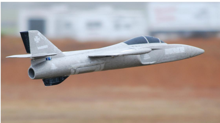
Quick foam pieces were added to a stripped, but stock Twister to assess changes that might improve handling qualities of the model during landing and stall.
